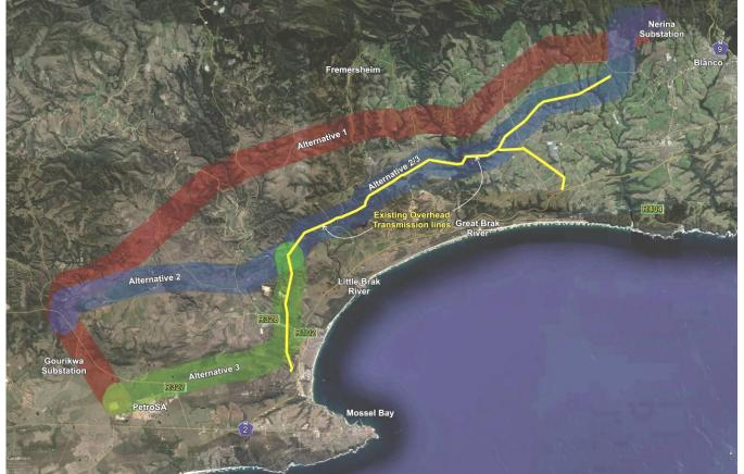
Figure 5: Proposed alternative route alignments shown in relation to the approximate alignment of existing overhead transmission lines through the study area (Source: GoogleEarth)
